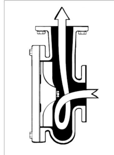
Vortex Design provides an unrestricted flow since the impeller is not normally in contact with the solids being pumped
